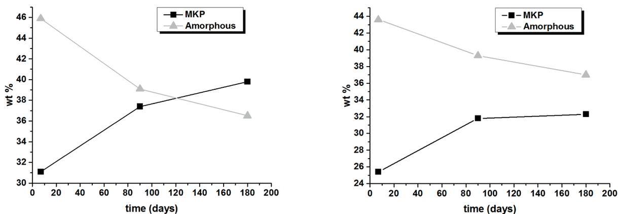
Fig. 2 Points corresponding to the phase fractions at different times of MKP and amorphous phase for the samples CHR\_1100 on the left (a), and CHR\_1300 on the right (b).
