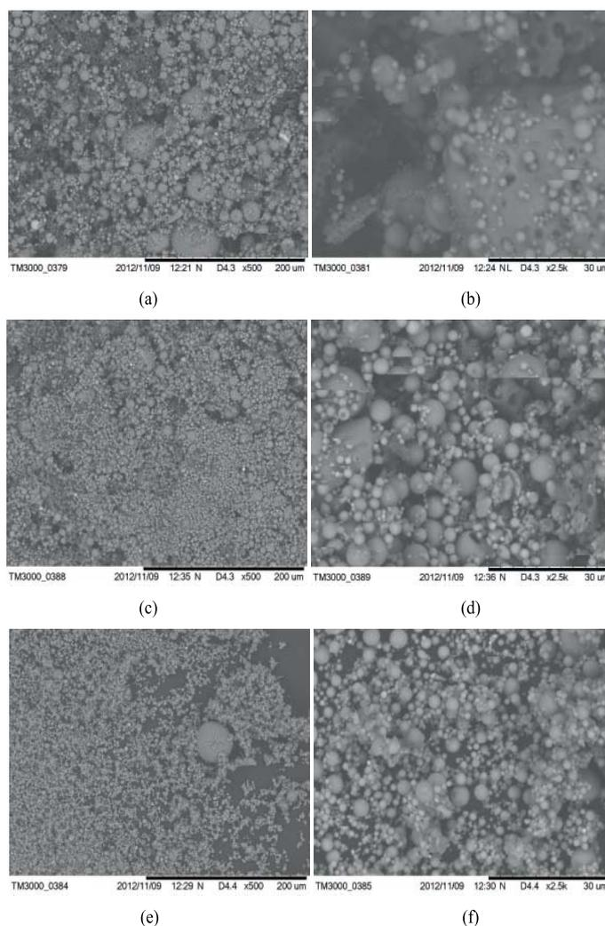
Fig. 1. Images of fly ashes: a, b) FA<sub>I</sub>; c, d) FA<sub>II</sub>; e, f) FA<sub>III</sub> zoomed 500x and 2500x.
