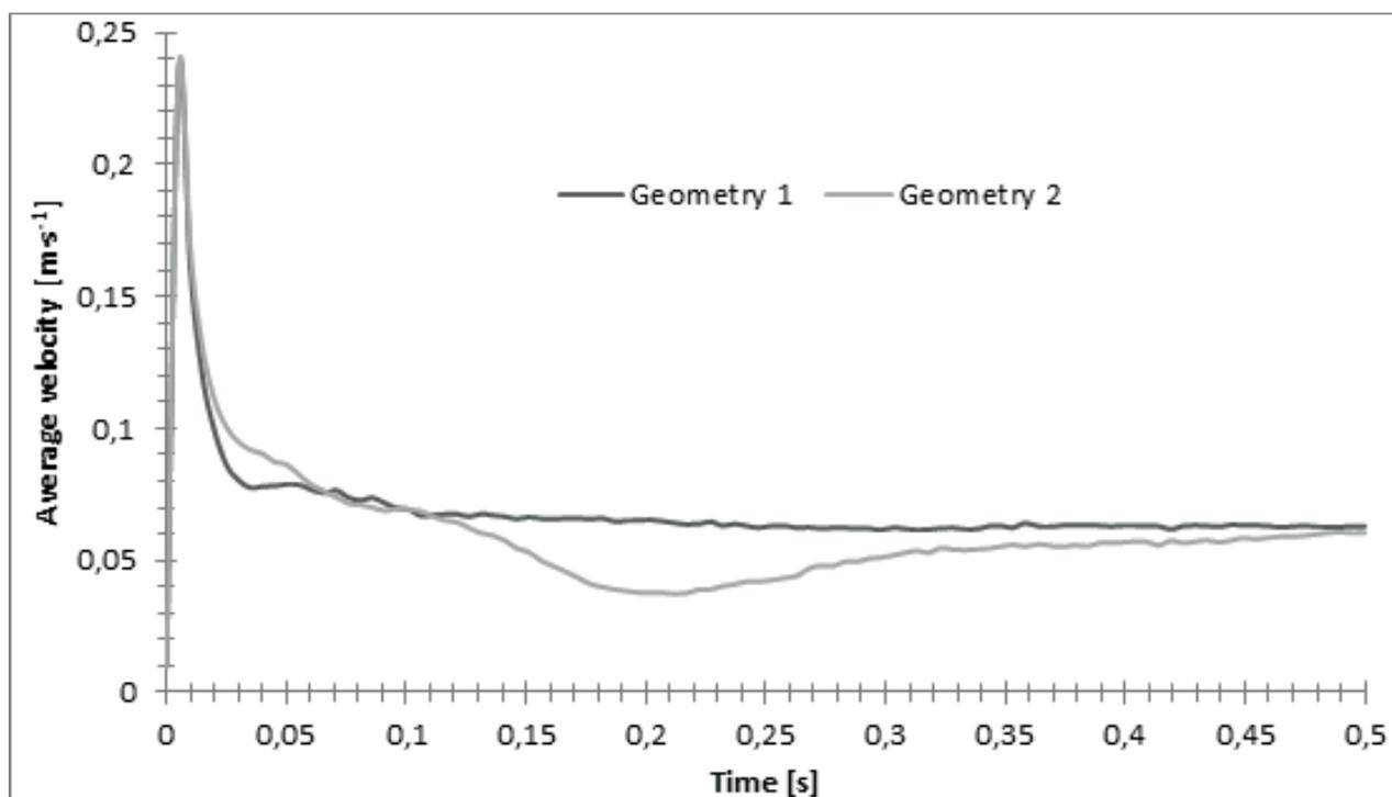
Fig. 6. The average velocity of the particles in the lowest scanning plane of conveyor
