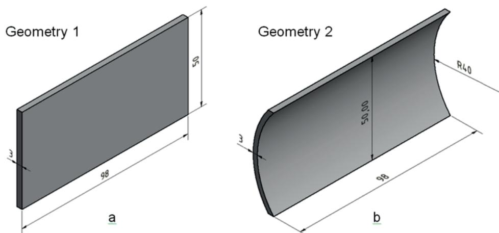
Fig. 2. Designs of the carrier geometry
