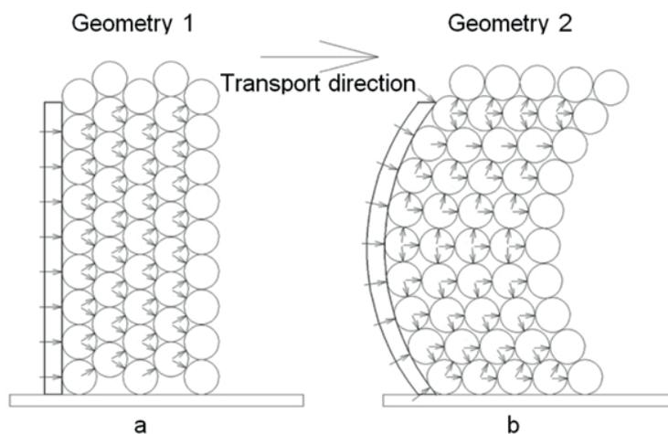
Fig. 3 Representation of spherically shaped particle contact surfaces occurring in the continuous flow of materials of the same type but with either of two alternative carrier geometries.
