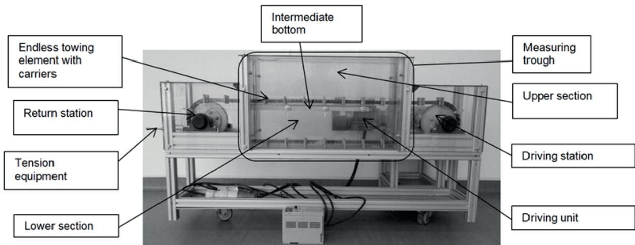
Fig. 1. The real model of the chain conveyor with carriers
