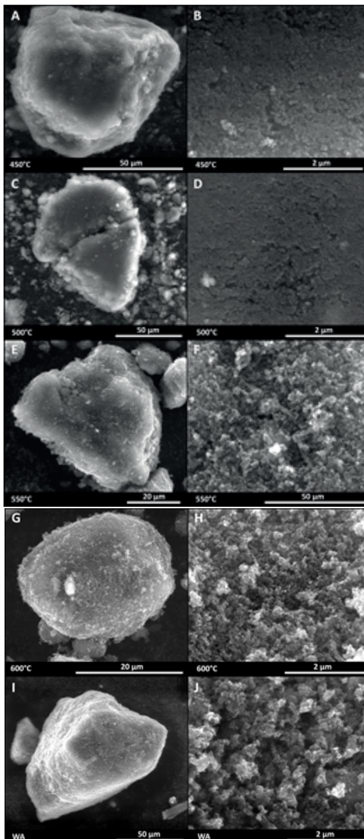
Fig. 2. Products of the pyrolysis at temperatures of 450°C (A, B), 500°C (C, D), 550°C (E, F), 600°C (G, H) and sample from industrial instalation (I, J). The secondary electrons (SE) images present development of active surface subsequent with increasing temperature conditions of pyrolysis
