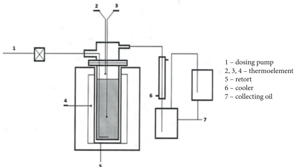
Fig. 1. Instalation for pyrolysis
