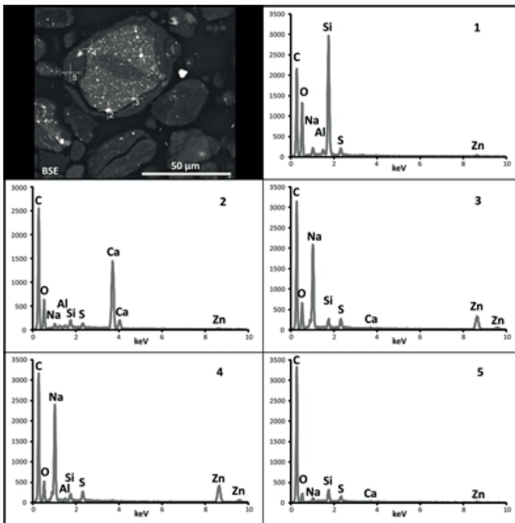
Fig. 3. Back scattered electrons (BSE) image presenting cross section of the polished sample with products of pyrolysis at 450°C. Si, Na and Ca-rich inorganic compounds form core enclosed in carbon shell. EDS spectrums represent chemistry of the analytical spots labeled 1–5 at the BSE image
