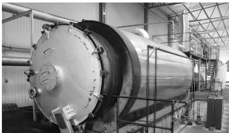
Fig. 1. Discontinuous pyrolysis plant XY-8 (batch process) of company Shangqiu Jinpeng Industrial Co., Ltd. – reactor or rather rotary pyrolysis kiln (photo – author)
