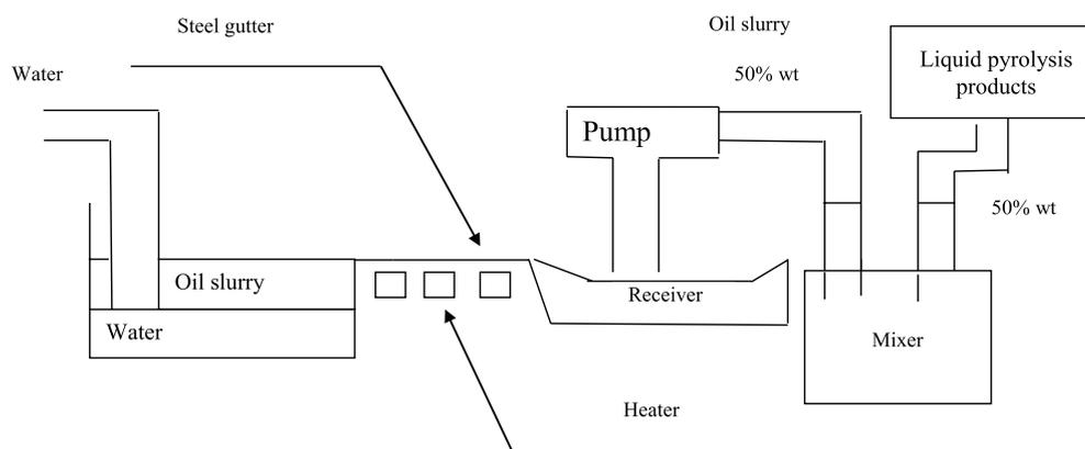
Fig. 1. Technological flowchart of the oil slurry excavation and liquefaction
