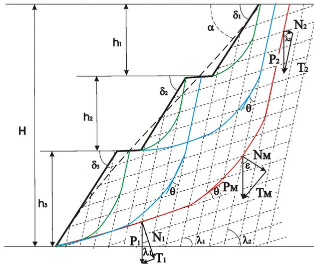
Fig. 1. Building slide surfaces in a cracked mass under the condition of shifting the landslip prism on cracks and mass
