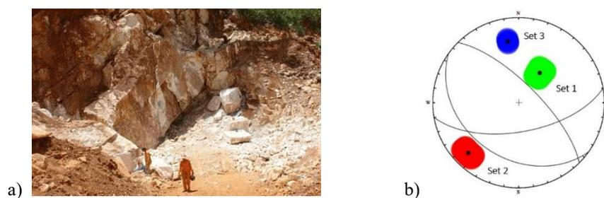
Fig. 6. Experiment pit M.01 (a) and 3 main joint sets of the Thung Khuoc quarry, Schmidt grid in hemisphere.
