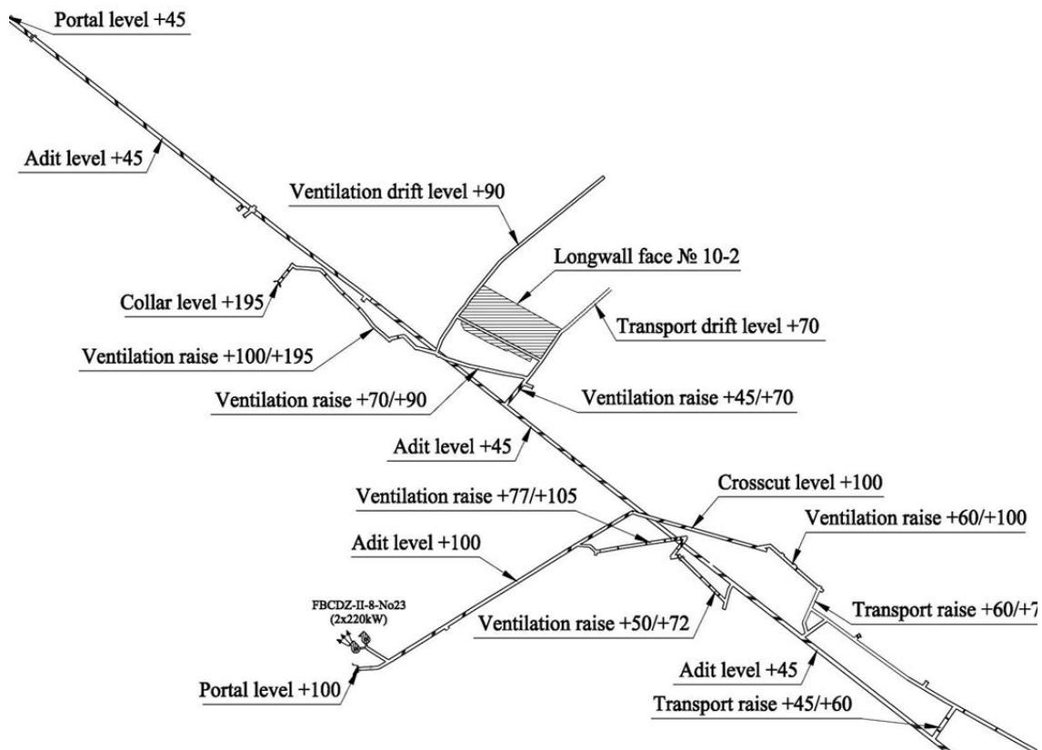
Fig. 1. Location of the longwall face № 10-2 at coal seam 10T, Company 86.
