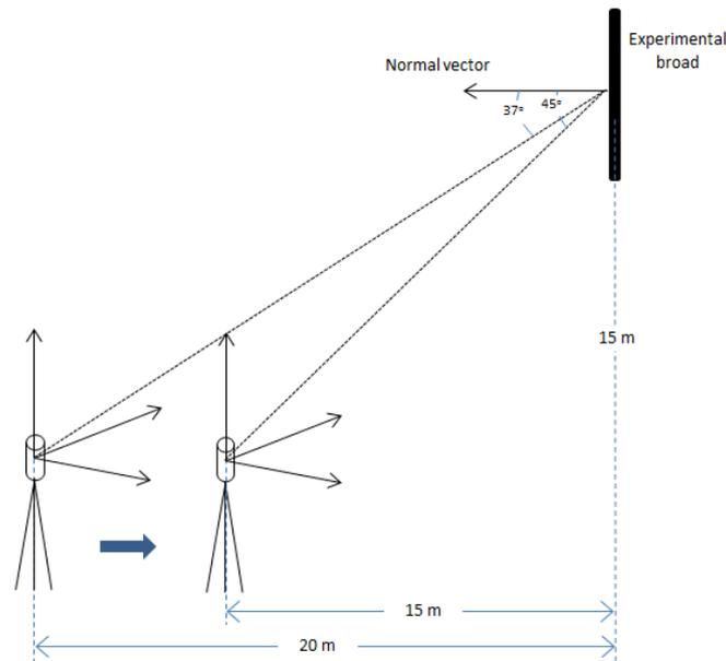
**Fig. 4.** Scanning geometry due to the incidence angle.
