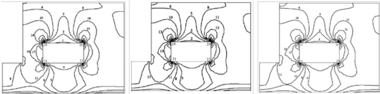
Fig. 2. Isolines of the principal stresses  $\sigma_1$  of the rock massif during creation of a horizontal compensation room in the panel: the pressure of caved rocks P1, ores with hardness a) 3–5, b) 4–6, c) 5–7 points respectively
