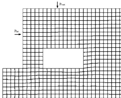
Fig. 1. Finite-element model with the horizontal compensation room
