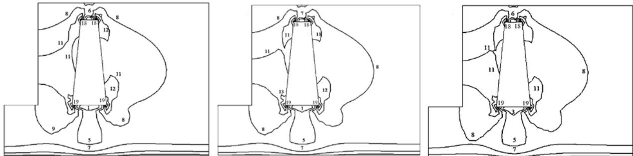
Fig. 3. Isolines of the principal stresses  $\sigma_1$  of the rock massif when creating a vertical trapezoidal compensation room in the panel: pressure of caved rocks P1, ores with hardness a) 3–5, b) 4–6, c) 5–7 points respectively
