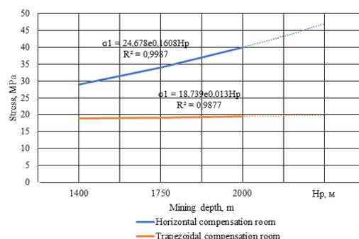
Fig. 4. Dependency of the value of the maximum principal stresses on the shape of compensation rooms and the depth of mining operations
