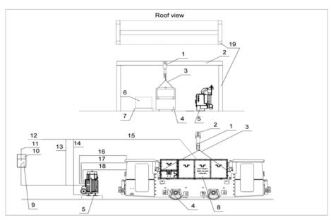
Fig. 2. Quick charging station on the ground (concept); 1 – self-propelled 6-ton chain hoist type SWŁ-6; 2 – running rail – l-beam 300 mm; 3 –
