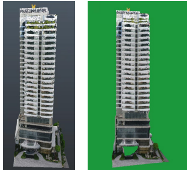
Fig. 8. Point clouds from UAV images
