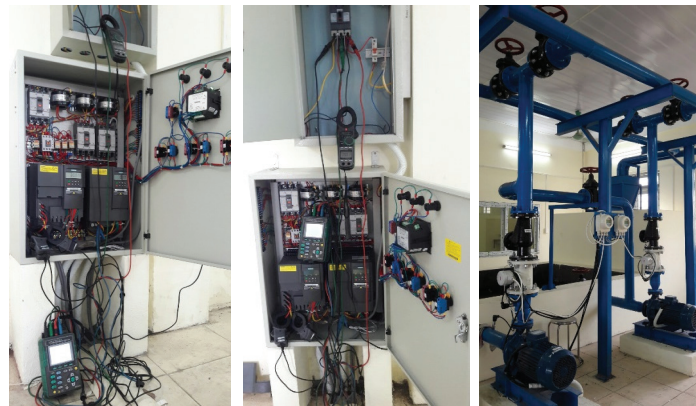
Fig. 11a. Lab-test setup for power losses measurement with pumping system
