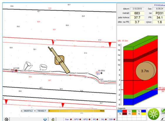
Fig. 9. Model GNSS Rkabina – GNSS extractor Cabin the current position and height of the excavator on the screen in the cab of the mining giant machine
