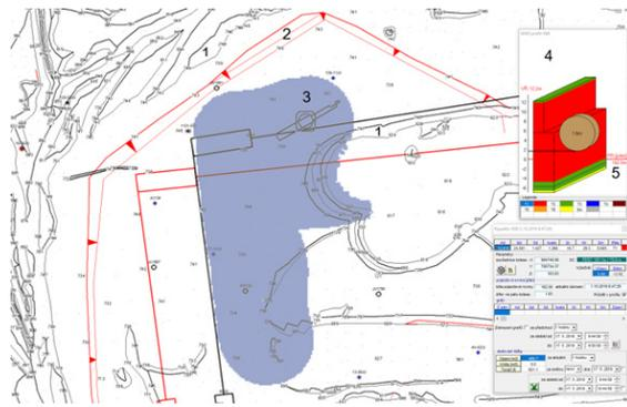
Fig. 11. Application "Technological model" for control and management of mining plan compliance – Bilina Mines, position of excavator K300.8/68 on 1 October 2019 at 8:47 AM
