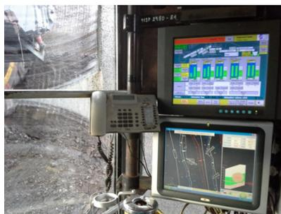
Fig. 10. The driver's cabin of the mining giant machine – on the right the screen with the "GPS cab" application
