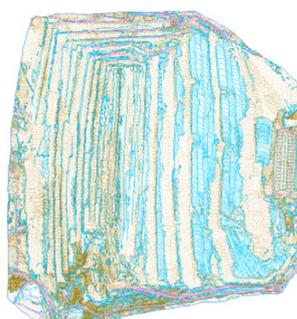
Fig. 3. Digital terrain model reduced to the active open pit mine area
